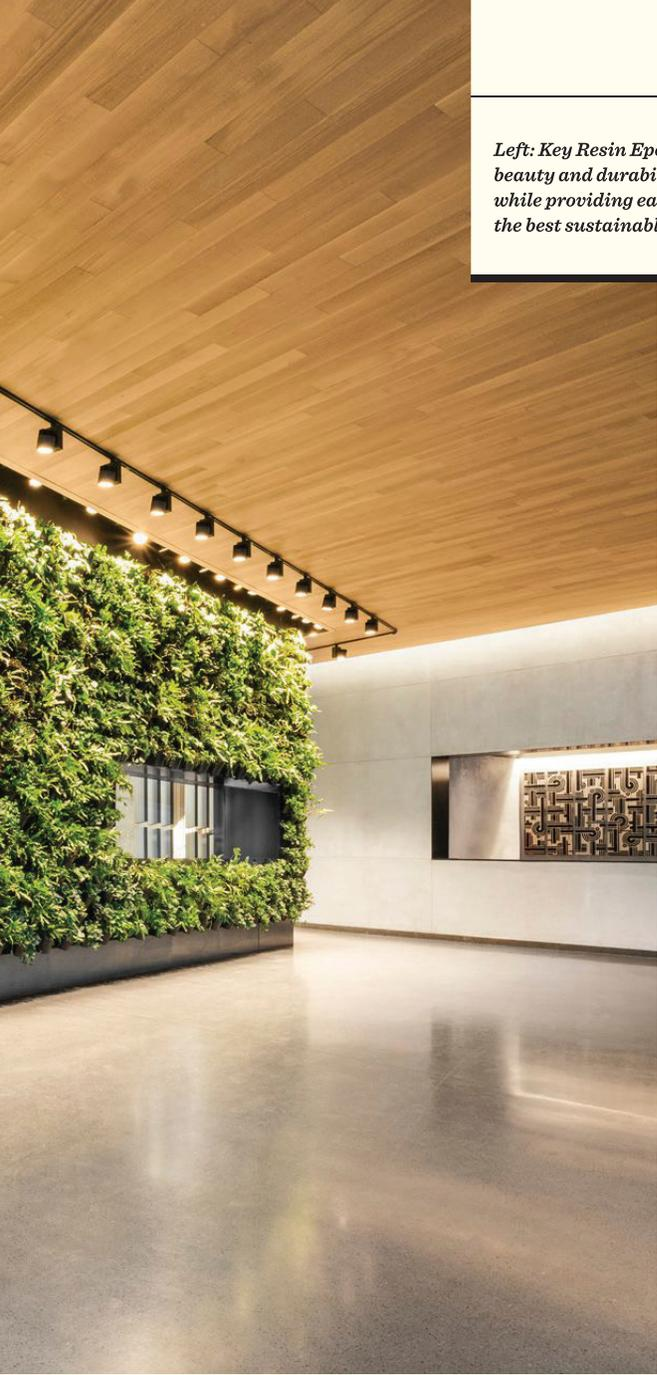
*Left: Key Resin Epoxy Terrazzo flooring delivers beauty and durability that lasts the life of the building while providing ease of maintenance consistent with the best sustainable building practices.*
